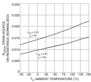
Fig. 6 On-Resistance Variation with Temperature
