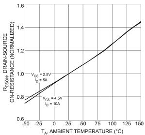
Fig. 5 On-Resistance Variation with Temperature
