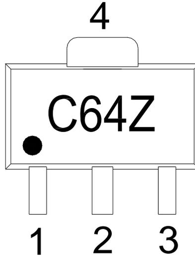
Alternate marking "SGC6489Z" on line one with Trace Code on line two.
