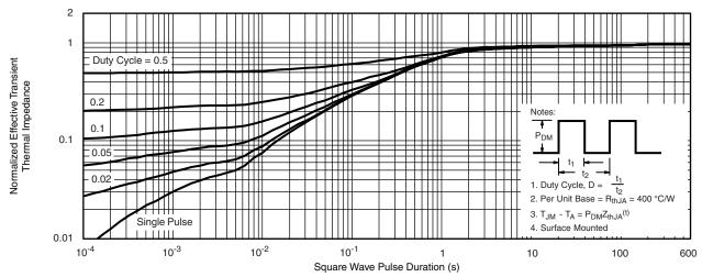
Normalized Thermal Transient Impedance, Junction-to-Ambient
