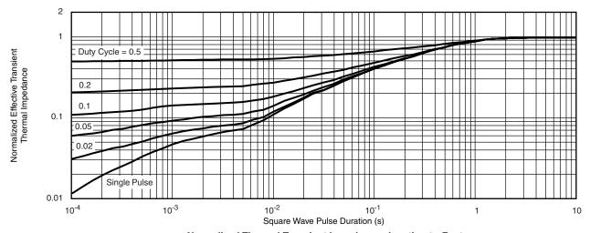
Normalized Thermal Transient Impedance, Junction-to-Foot
