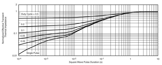
Normalized Thermal Transient Impedance, Junction-to-Foot
